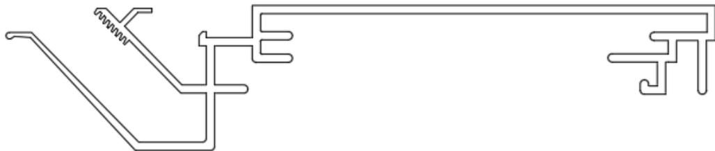
**6.2. Figure below shows the cross-section of the side body section simplified to allow conservative calculation of the sectional properties**
